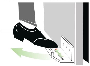
Important! StepNpull® will work great on any commercial solid core wood door or commercial metal door regardless of the door's size or weight. If, however, the door is abnormally difficult to pull open, the door closer resistance should be decreased.
